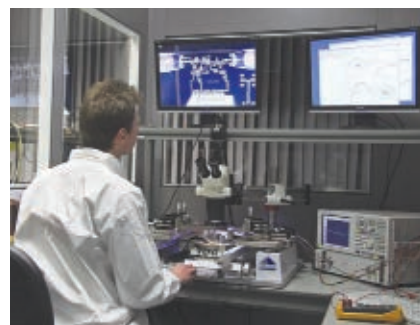
▲ Fig. 2 Evaluation of a mm-wave amplifier MMIC in Plextek's RFW test laboratory.
